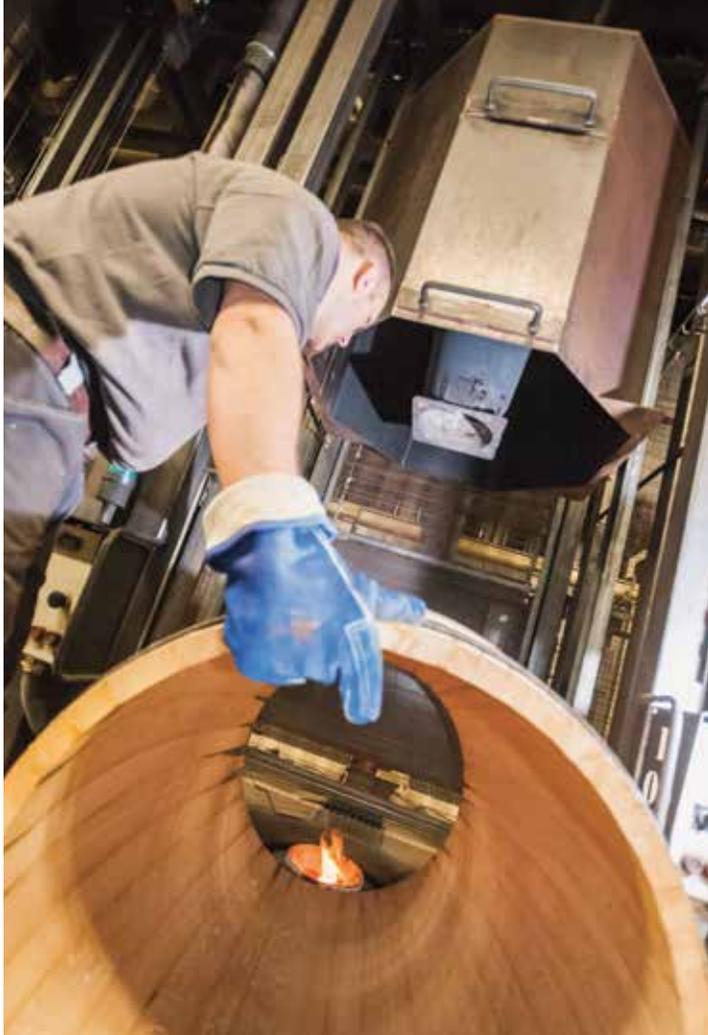
The toasting system has an inner cone covering the flame and an outer dome that eliminates environmental fluctuations.
